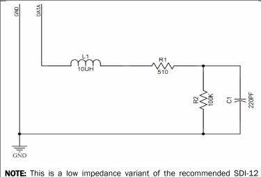
Specification. This allows up to 62 sensors to be maintained on a bus.
